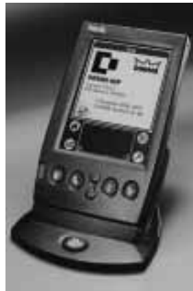
Handheld computer for servicing and commissioning with DORMA Automatic Service Program (ASP)
